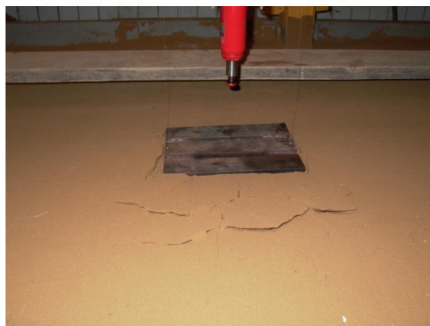
Figure 2.9 Propagation of fissures in soil [G.G. Boldyrev, A. (2008)]
