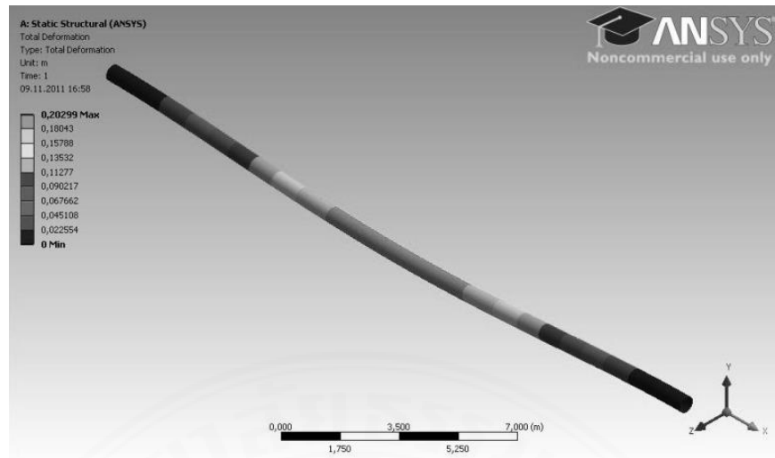
Figure 2.15 Deformation contours of pipeline [Burkov, PV (2014)]
