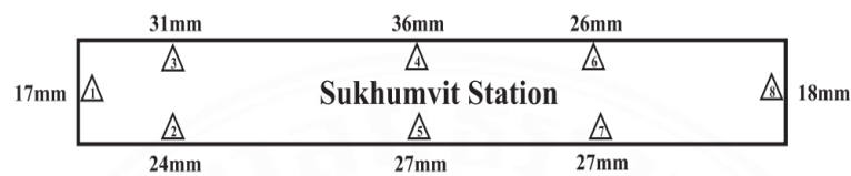
Figure 2.3 Maximum horizontal movement of D-walls [Likitlersuang, S. (2013)]
