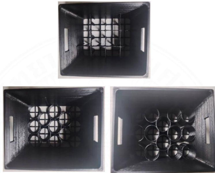
Figure 5.3 Prototype of three-crate design (with the size of 20% from full actual version): (a) original crate, (b) crate-assembly and (c) crate-fourteen.
