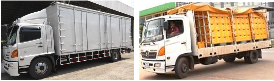
(a) Comparison between two styles of vehicle – rigid closed truck and opened truck.
