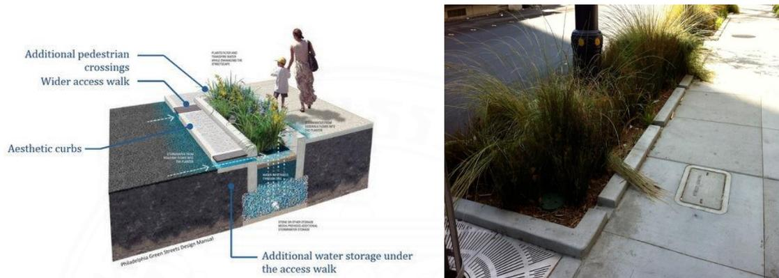
**Figure 2.8** Cross-sectional view of a bioswale design and example of curbside bioswale in practice. Retrieved from (<https://www.reliance-foundry.com/blog/bioswale-design>)
