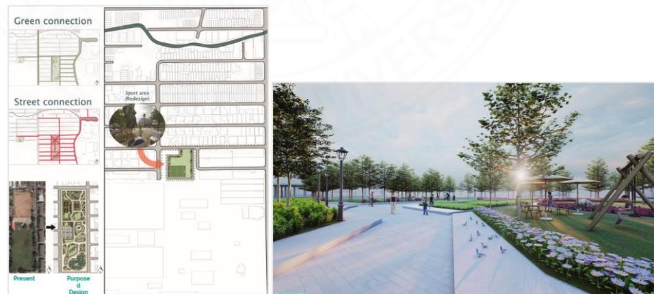
**Figure 3.16** Example of gardenland park design (referred as raingarden in the study) for a vacant land area represented as subcatchment 104 in the model (designed by Tanavara, T., Paveena, K., Manita, I., Yuto, M.)
