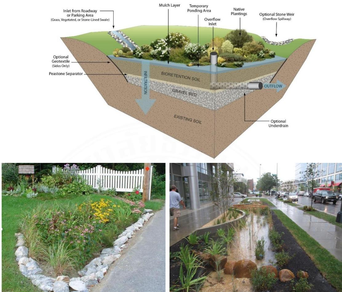
**Figure 2.7** Schematic representation of bioretention cell design (above) and examples of this application (below) for the residential area (left) and pedestrian roadway (right). Retrieved from (<https://megamanual.geosyntec.com/npsmanual/>)
