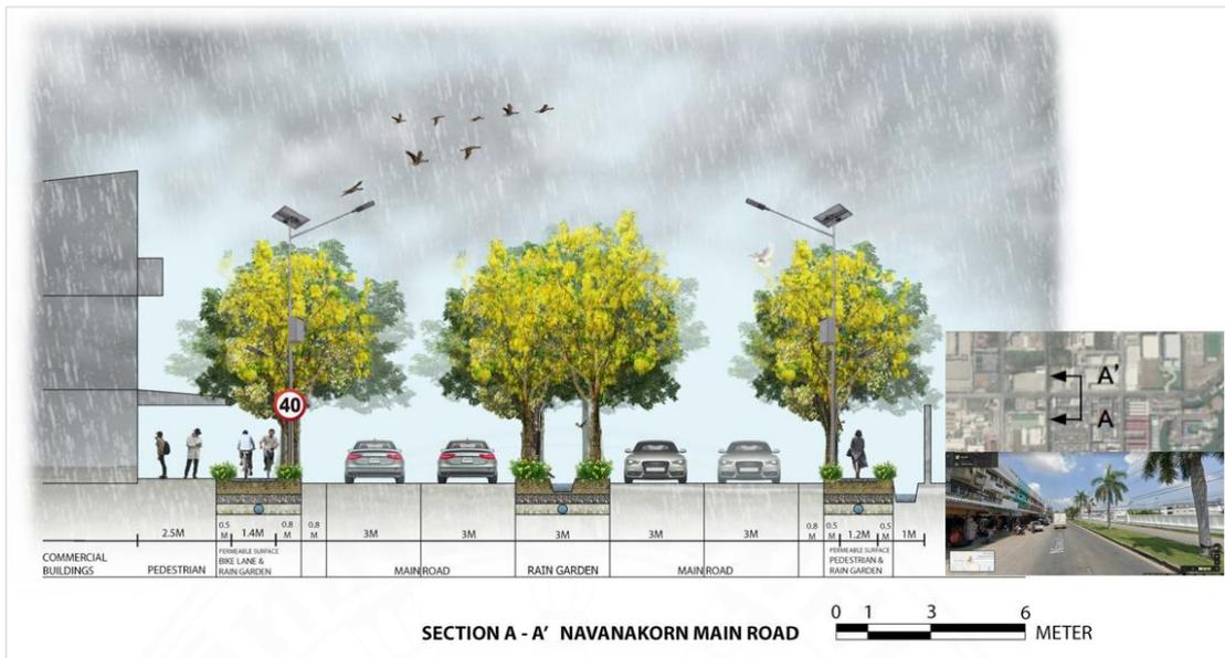
Figure 3.10 Cross sectional view of a typical raingarden for the major road inside Nava Nakorn or section A'A
