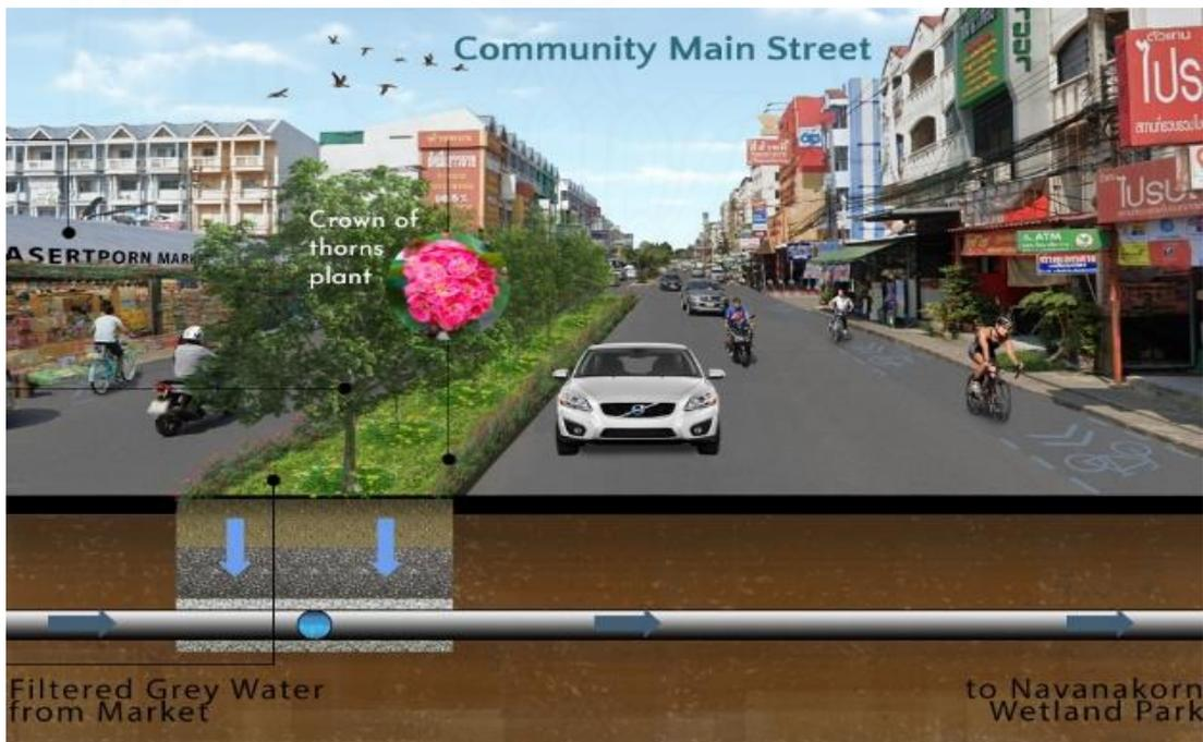
Figure 3.11 Bioretention cell design on the community main street (section B'B) with underdrain illustrated as in streetscape view (Designed by Tanavara, T., Paveena, K., Manita, I., Yuto, M.)
