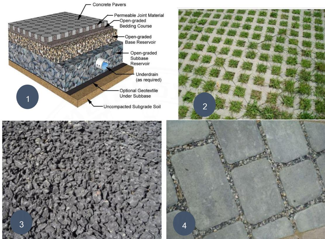
**Figure 2.6** Schematic representation of permeable pavement (picture 1) and some examples of the permeable pavement surface (picture 2, 3, 4). Retrieved from (Freeborn et al., 2015)
