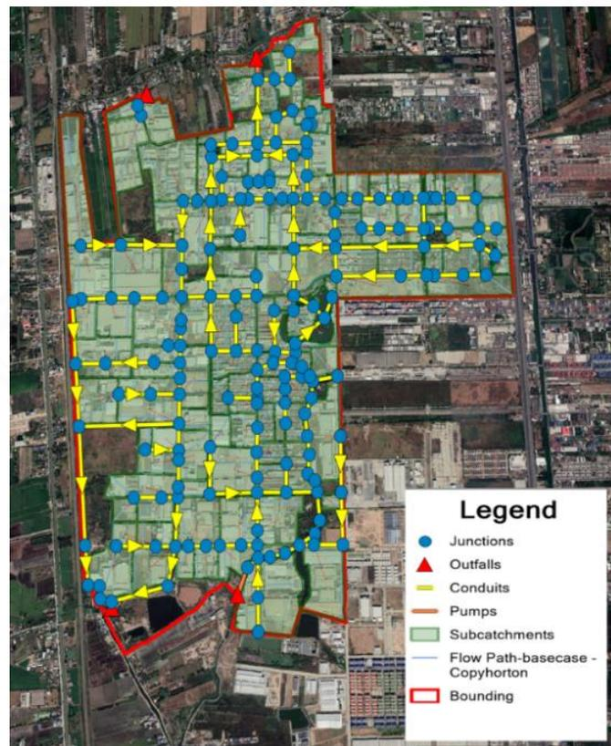
Figure 4.1 PCSWMM configuration for the runoff and drainage systems inside Nava Nakorn
