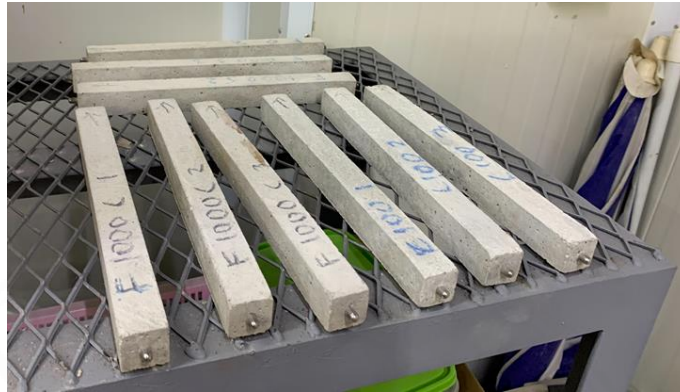
Figure 3.5 Total Shrinkage specimens.
