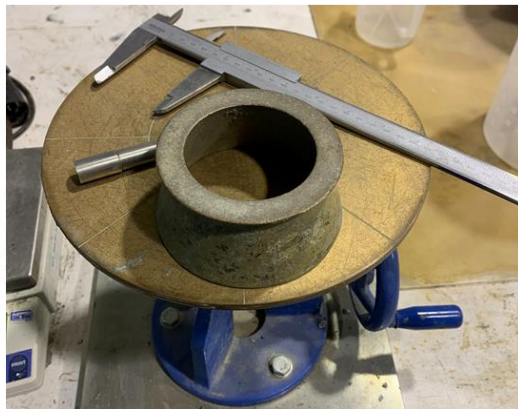
Figure 3.2 Flow tables, flow cones, tamping rod, and vernier caliper
