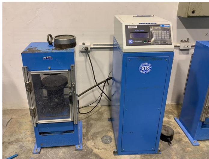
Figure 3.3 Compressive strength test machine.
