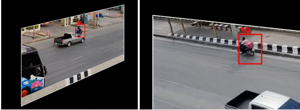
Figure 6.6 The screenshots when capturing vehicles driving in the wrong direction in the vertical oriented video.
