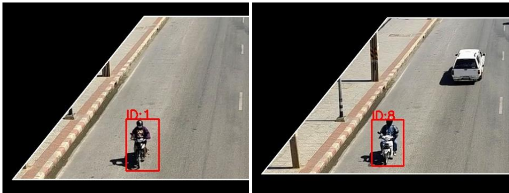
Figure 6.4 The screenshots when the CY bounding box is above YL by 20 pixels.
