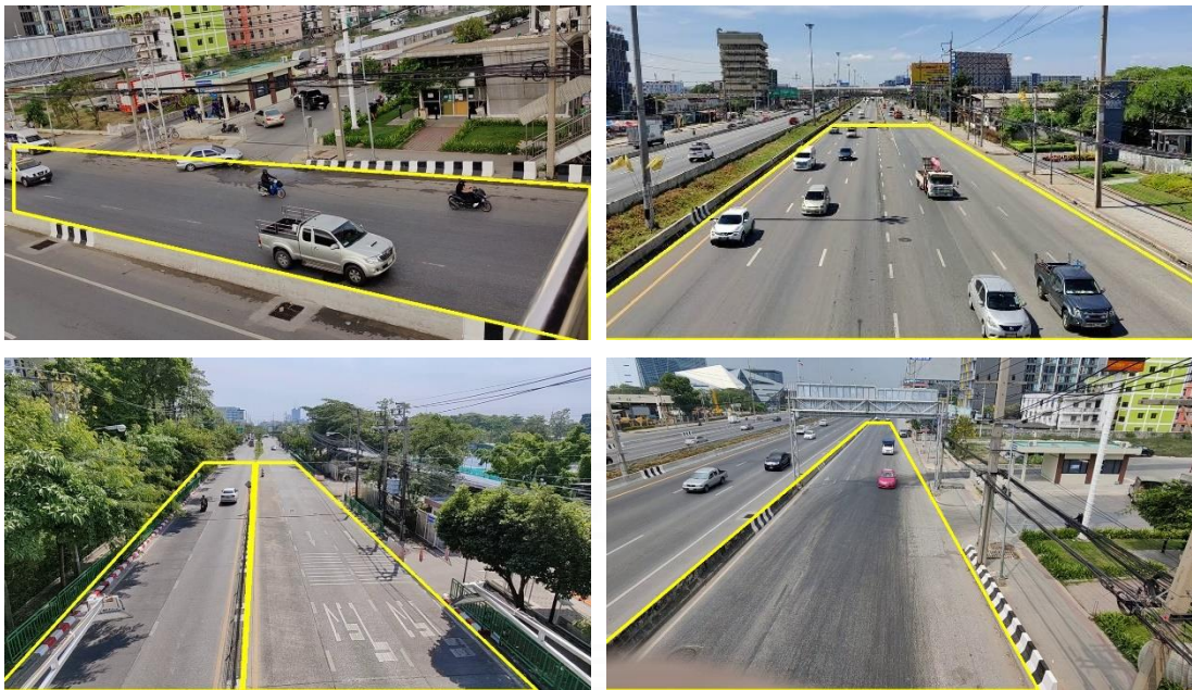
Figure 7.2 Output images with road boundaries using the RLB-CCTV algorithm.
