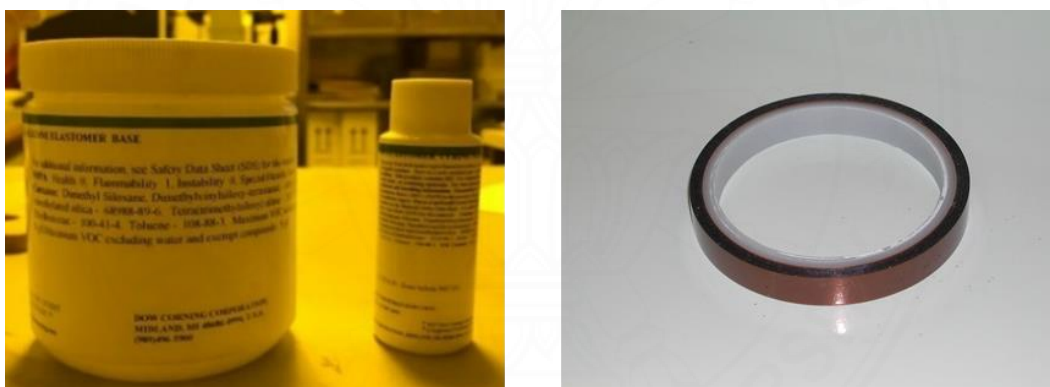
Figure 3.4 The PDMS precursor together with its curing agent (left) and the polyimide tape used in this work (right)
