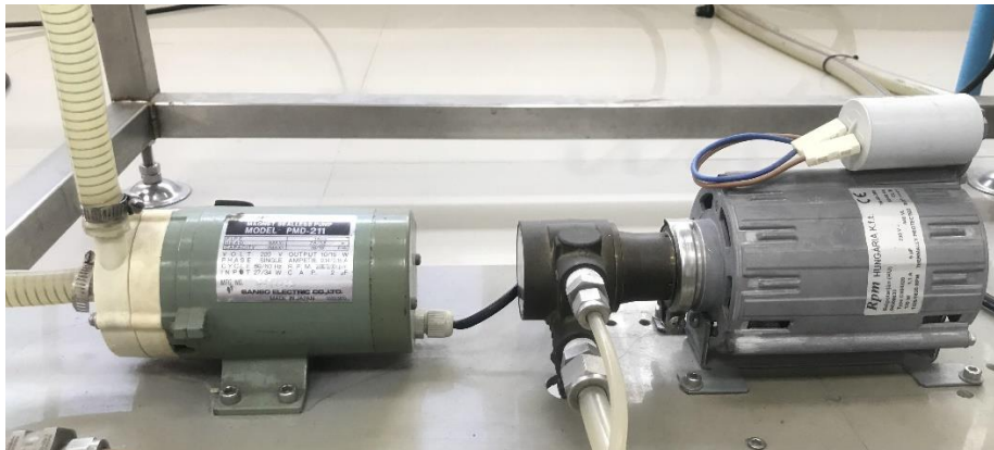
Figure 4.9 The evaporator recirculating pump and the boiler feeding pump
