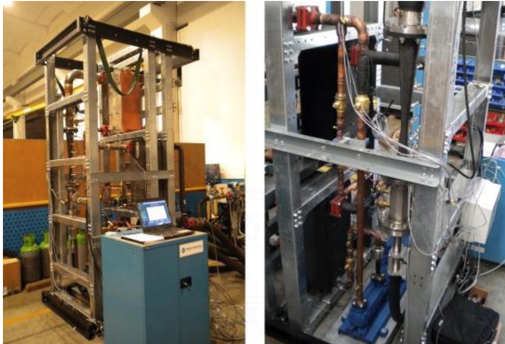
Figure 2.15 A R245fa ejector refrigerator operated as a chiller machine developed Eames et al. (2013)
