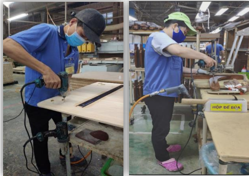
Figure 3.2: Performing task with drilling and screwing
