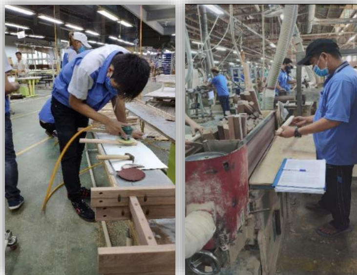
Figure 3.1: Two types of sanding exposure to vibration
