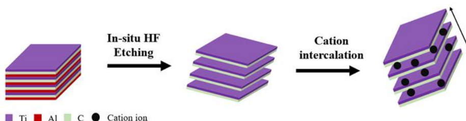
Figure 4.1 Schematic illustration of the in-situ HF etching of the MXene ( \text{Ti}_3\text{C}_2\text{T}_x ) material.
