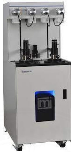
Figure 3.12 Micromeritics AutoPore 9600 machine for MIP test (micromeritics.com, 2015)
