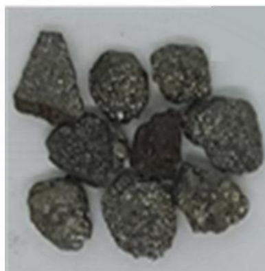
Figure 3.3 Tested iron sulfide-containing aggregates (Saengsoy et al., 2021)
