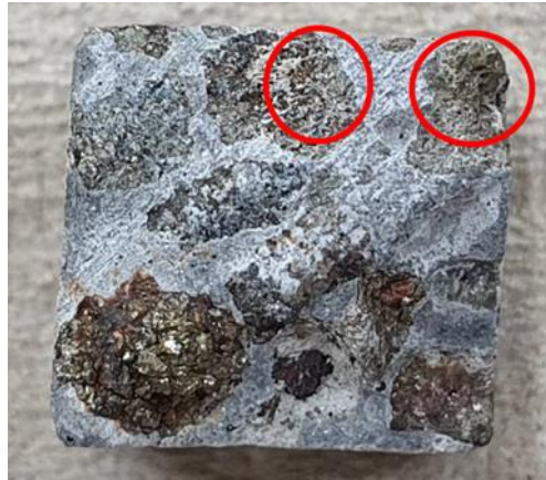
Figure 4.4 Cut mortar bar (FAM30) used to do SEM (before coated with gold)
