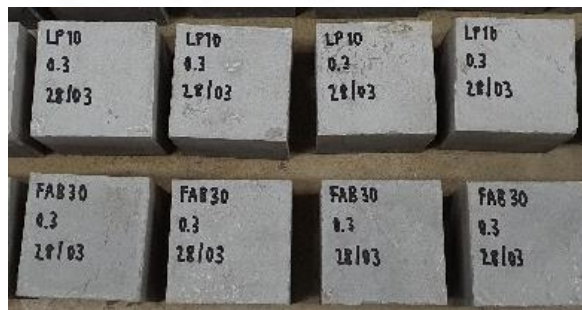
Figure 3.9 Cement paste cube (after demolded) used for TGA/DTG and MIP tests
