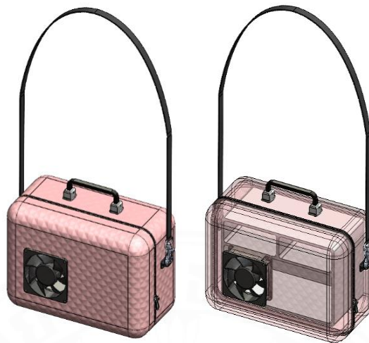
Figure 3.11 Main Components of The Carry-On Bag – Design D, (Left) Isometric View, (Right) Transparent Display Of Isometric View.
