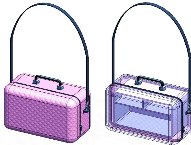
Figure 3.7 Original Design Of “Design C” – Carry-On Bag Inspired from Classic Briefcase Baggage – Design B, (Left) Isometric View, (Right) Transparent Display of Isometric View.
