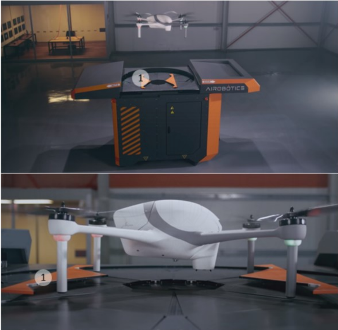
Figure 2.3 Commercially available positioning platform which use four V and W shaped pushers
