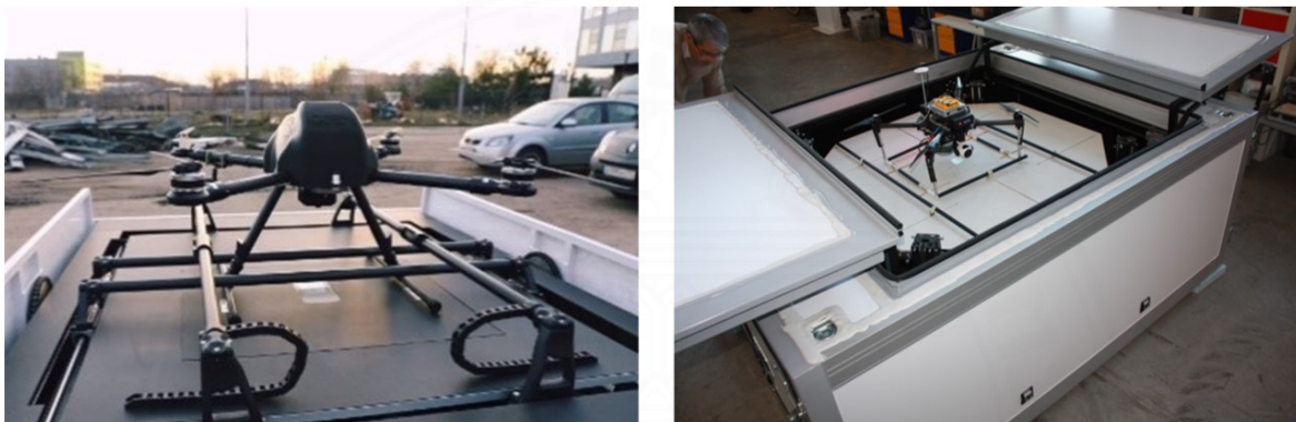
Figure 2.2 Commercially available positioning platform which use four parallel pushers
