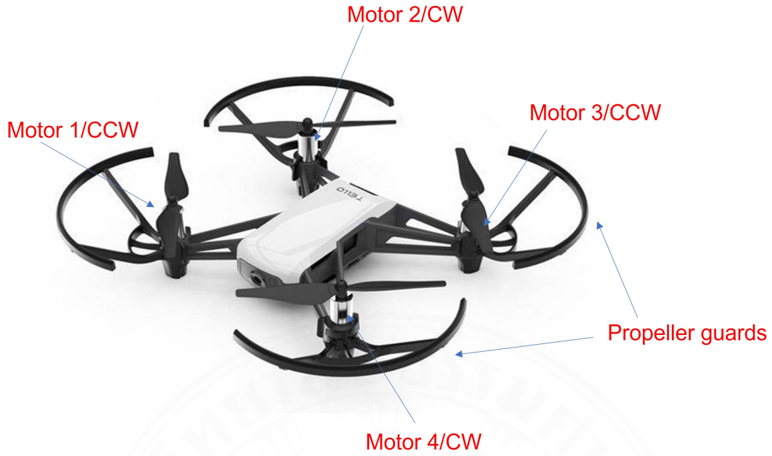
Figure 3.5 DJI TELLO quadrotor UAV used for the experiment
