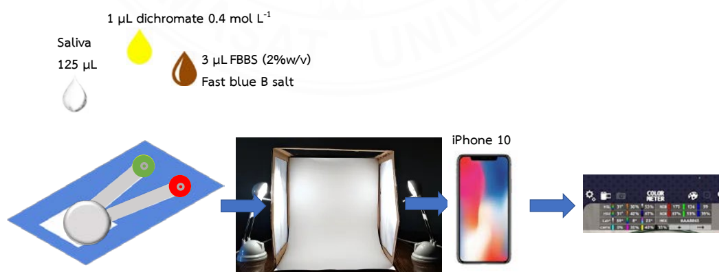
Figure 3.10. The operation of a proposed microfluidic device for colorimetric detection of ethanol and THC in a synthetic saliva sample.
