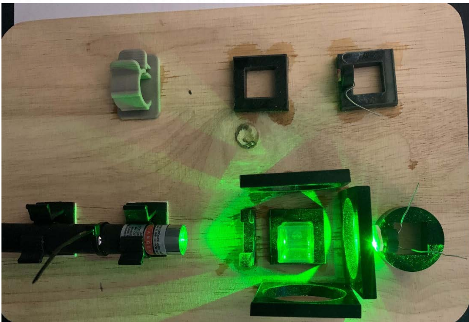
Figure 4.3. The design and invention of the green laser-LDR spectrometer.
