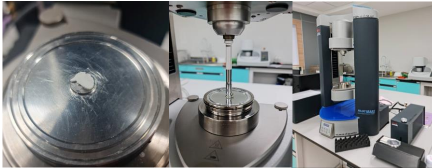
Figure 3.4 Sample preparation for viscosity testing.
