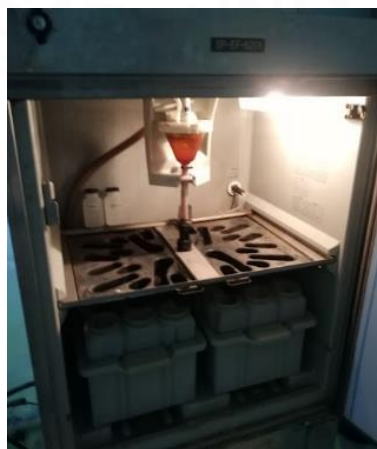
Figure 3.3 Automatic Wastewater Sample Collector.
