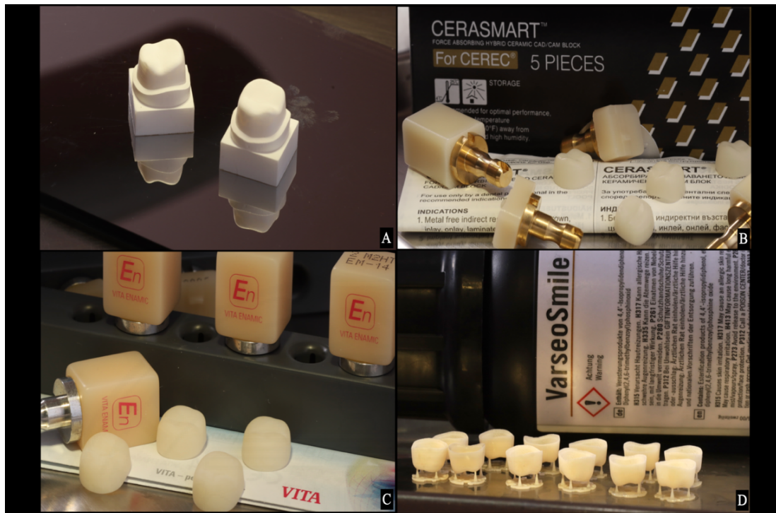
Figure 3. CAM fabrications of specimens; Rigid 10K resin dies (A), Cerasmart® milled crowns (B), Vita Enamic® milled crowns (C), Varseosmile® 3D-printed crowns (D)
